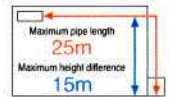
SRK50ZGX-S For an installation involving piping that measures more than 15m but no more than 25m, add R410 refrigerant at a charge rate of 20g/m.
